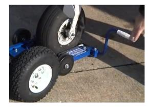
For unloading, chock the aircraft wheels. Release the Open/Close Latch to allow the swing gate to open and pull the tug away from the aircraft.
